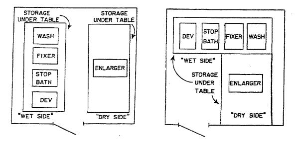
Figure 5-1. Two examples of laying out a darkroom.
