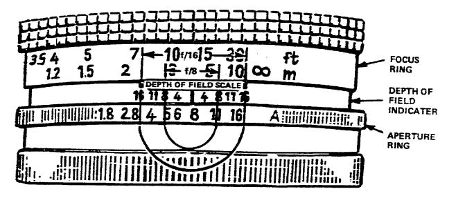
Figure 1-2. Depth of Field Scale
